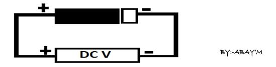
**Reverse Biasing:** - applying positive (+) DC to cathode and (-) DC to anode so in this case positive charge of battery attract anode of diode in other way negative charge of battery attract cathode of diode in turn making the gap wide. So current can not flow.
