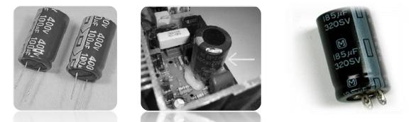
**Function of Electrolytic capacitor**:- **DC filter** rectified signal by diodes isn't pure it has ripple. Capacitors avoid these ripple electronic capacitors avoid these ripple.
