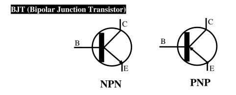
There are two configurations for a common **BJT** transistor: NPN (negative-positive-negative) and PNP (positive-negative-positive).Notice the difference symbols for NPN and PNP transistor. The emitter arrow points away from the transistor body for an NPN and toward the transistor body for PNP.
