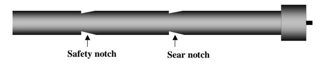
With the notches cut, the striker can be re-fitted and the weapon is ready to test fire.
