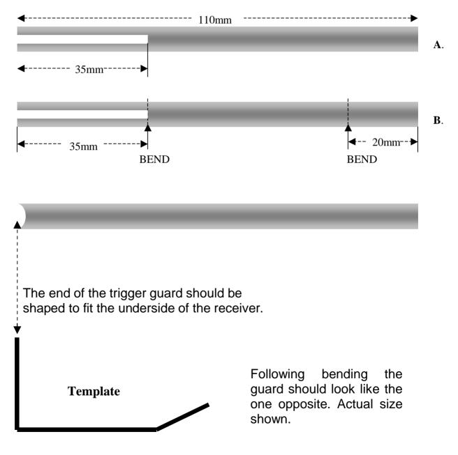
With the trigger guard finished it is ready to be welded to the receiver. A slot may be cut into the front of the grip to accommodate the end of the guard.
