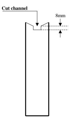
After cutting the curved groove across the top of the grip a square channel can now be cut to accept the trigger bar.
