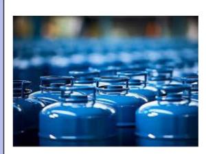
LPG is a product obtained during the processing of natural gas or the refining of crude oil It is composed of various hydrocarbon gases, with propane (C3H8) and butane (C4H10) being the primary components which have the property of being gases at normal ambient temperature but can be liquefied and kept in the liquid state by quite moderate pressure. In comparison with traditional fuels, LPG can be up to five times more efficient.
