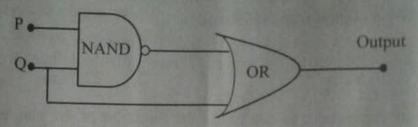
The truth table for the logic circuit shown above is
