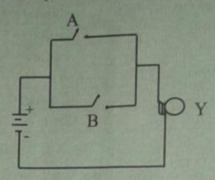
Which one of the following logic get can be represented by equivalent switch circuit?
