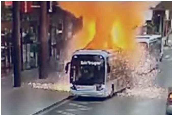
Figure 6 - Example of Thermal Runaway in roof mounted batteries involving a hybrid Paris Bus on 19.04.2022
