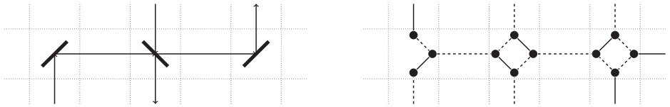
Figure 15.2 Reduction of the laser problem (left) to a perfect matching problem (right). The matching edges are shown with solid lines.
