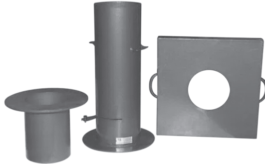
Fig. 4.1: In situ density by sand replacement method (Courtesy: AIMIL Ltd.)
