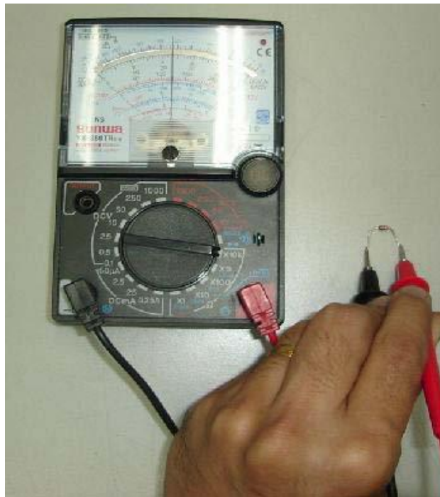
Use analogue multimeter to test zener diode
