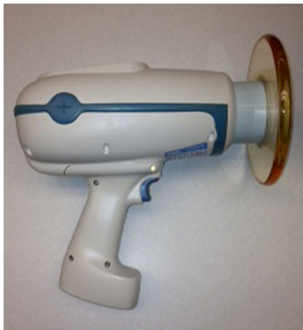
Fig. 6.3 NOMAD® handheld portable radiograph unit (Photo of actual equipment)
