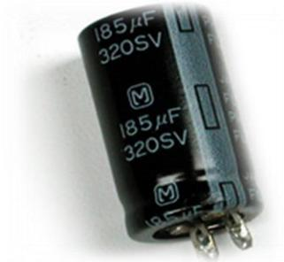
**Function of Electrolytic capacitor:-** DC filter rectified signal by diodes isn't pure it has ripple. Capacitors avoid these ripple electronic capacitors avoid these ripple.
