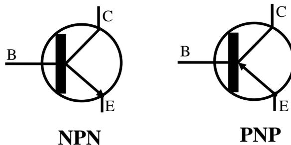
There are two configurations for a common **BJT** transistor: NPN (negative-positive-negative) and PNP (positive-negative-positive). Notice the difference symbols for NPN and PNP transistor. The emitter arrow points away from the transistor body for an NPN and toward the transistor body for PNP.
