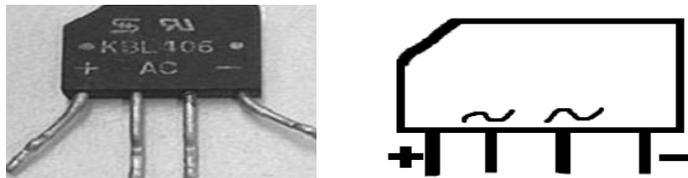
As shown bridge IC can be used instead of four diodes. The two inner terminals are where AC signals input where as the end two legs are terminal where rectified output obtained.
