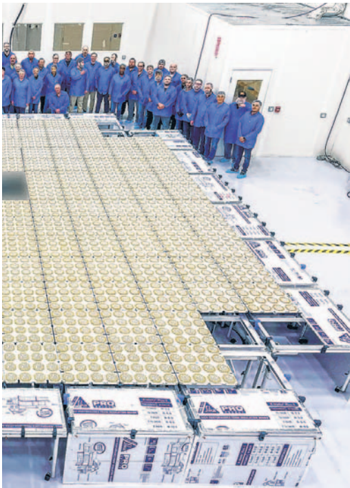
AST SpaceMobile staff stand behind the Micron panels that were later assembled into a satellite's phased array. The satellite was used to conduct voice calls, data downloads, videocalls, and streaming video playback from unmodified phones connected directly to a satellite in space using terrestrial cellular frequencies.
